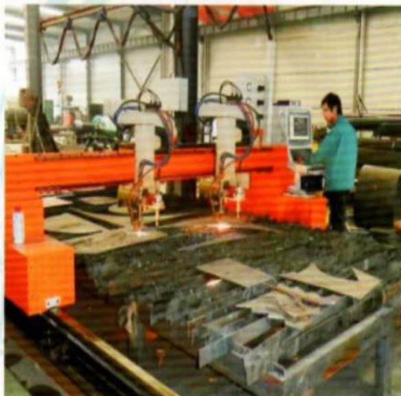
YH-300DHD 数控等离子/火焰两用切割机 CNC plasma/flame and cutting machine
